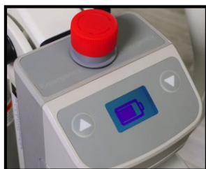
LCD battery level display; audible low-battery indicator
